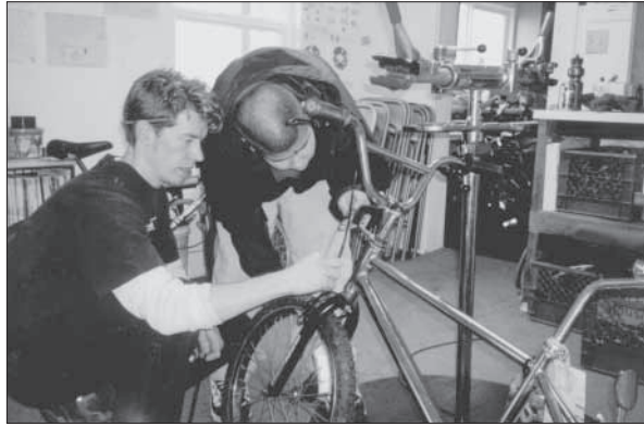
Chris and Hiram adjust the brakes on a BMX-style bike.
