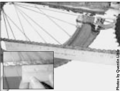
Use a ruler to measure the wear of the chain.
